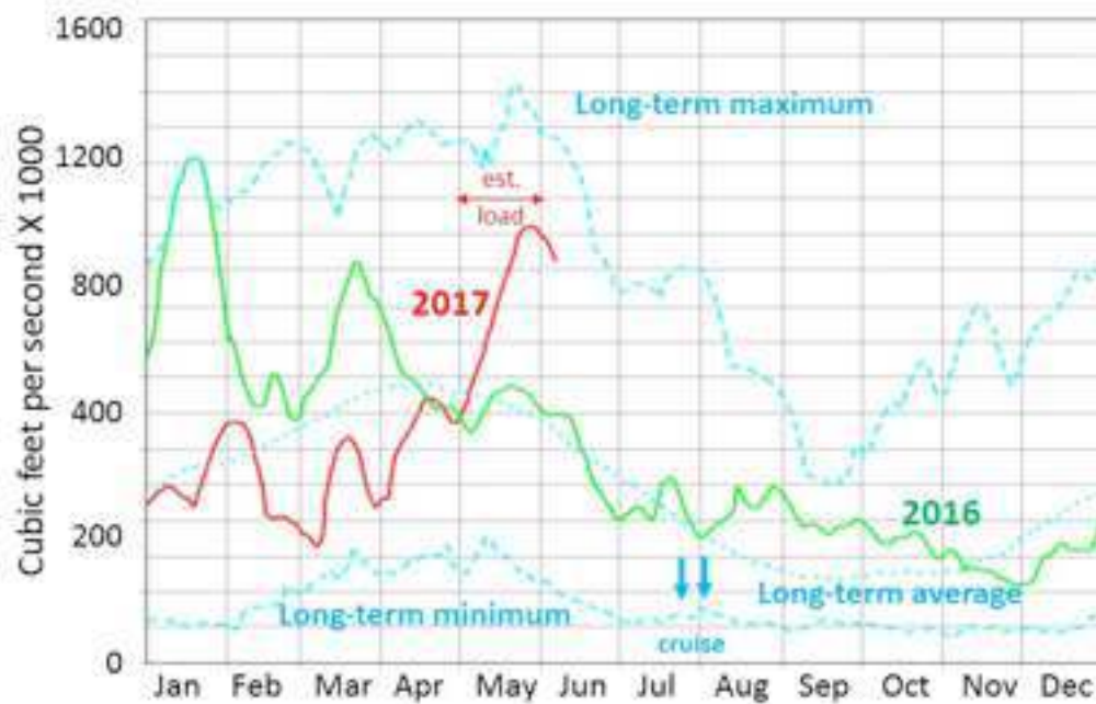
Appendix Figure 2. The daily river discharge at Tarbert Landing, LA, from 1935 through 1 Jun 2017. Units are cubic feet per second \times 1000. The period of the nitrate load is shown with a red horizontal arrow; the timing of the summer hypoxia cruise is indicated by the blue vertical arrows. Figure modified from http://rivergages.mvr.usace.army.mil/WaterControl/Districts/MVN/tar.gif .
