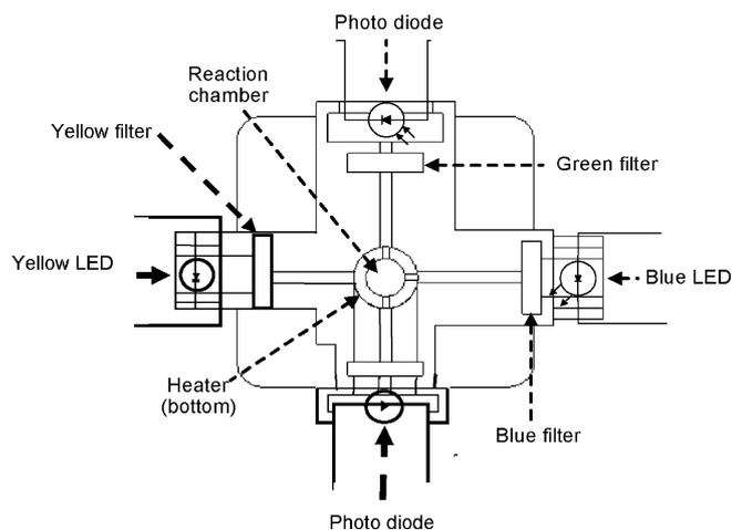
Fig. 1. Schematic diagram of the handheld NASBA analyzer.
