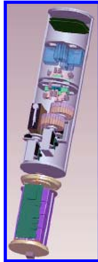
Figure 2. Schematic of a prototype Autonomous Microbial Genosensor (AMG), a NASBA-based amplification and detection platform.
